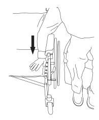
NOTE: Press down on the seat rail and the seat upholstery with the entire hand. DO NOT place any part of the hand under the seat rail.
